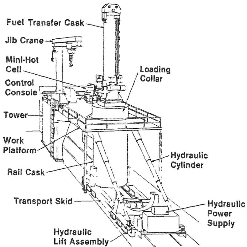
Figure 4. Schematic of the NuPac 125-B rail cask being loaded with a core debris canister at TMI-2, using the shielded fuel transfer cask.
