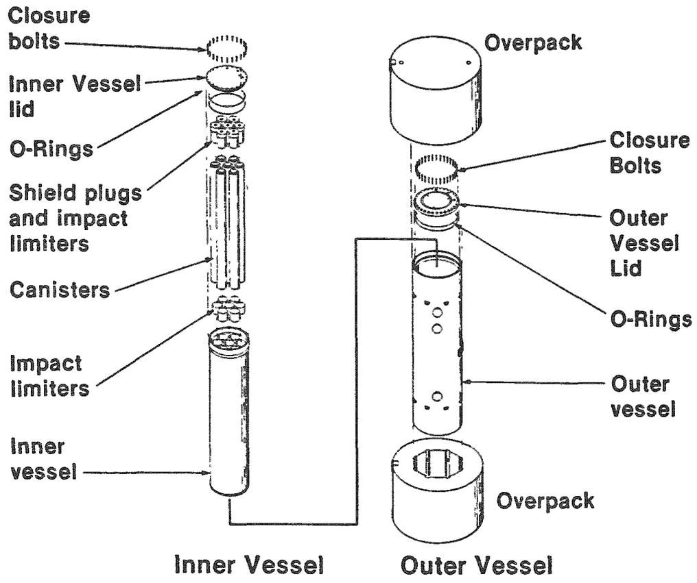
Figure 2. Disassembled view of NuPac 125-B cask.
